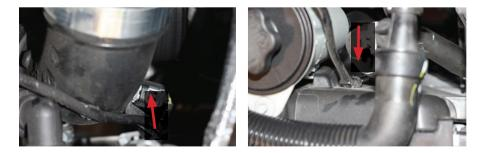
Remove the bolt holding the power steering reservoir to the fan shroud. Pull the power steering reservoir up to disconnect it from the fan shroud and just let the reservoir swing free to temporarily provide easier access to the lower intercooler pipe connection point (on intercooler). Loosen the lower factory t-bolt clamp (at intercooler).
