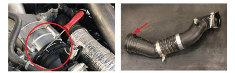
Twist carefully **(1/4 turn counter-clockwise)** to unlock and remove the intake air temperature sensor from the factory plastic throttle body coupler. Apply some vaseline or grease to the o-ring of the factory intake air temperature sensor and install it into the machined port on the supplied HSM billet aluminum throttle coupler. Be sure to carefully twist the sensor to properly lock it into place **(1/4 turn clockwise)**.
